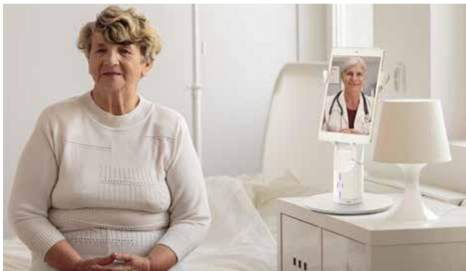
*Kubi telepresence robot features a stationary base and arms that hold a tablet computer. A remote user can tilt or pan the tablet using these arms to gain a different camera view. Image courtesy of Xandex, Inc.*
