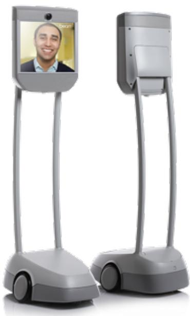
*Beam® by Suitable Technologies® is a telepresence device that offers 'videoconferencing with mobility.' Image courtesy of Sustainable Technologies*
